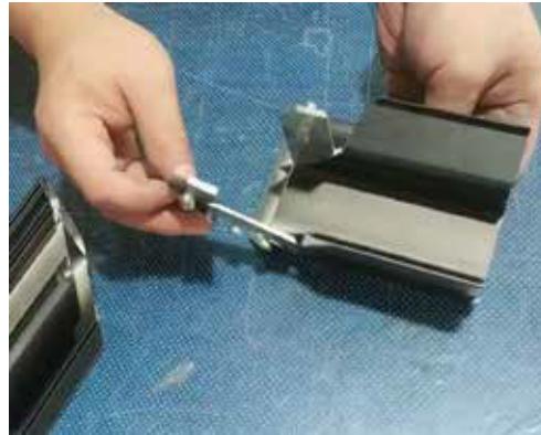
Insert the L shape connector
